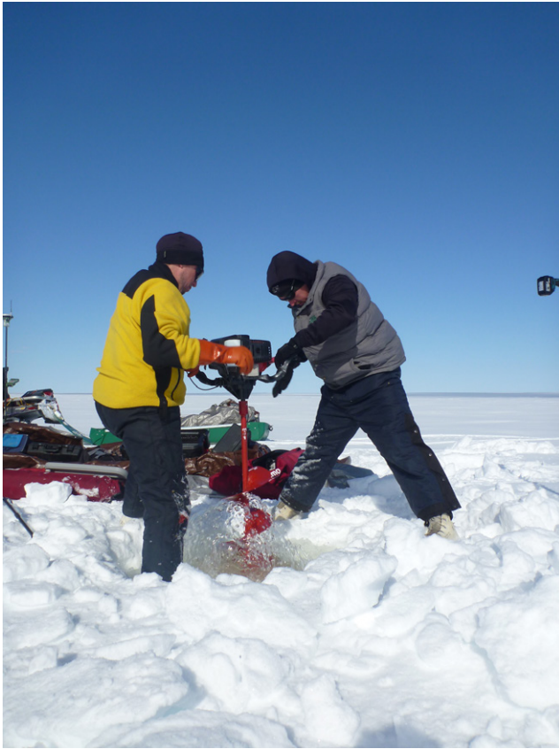
Christopher Arp and Benjamin Jones auguring a hole in the lake ice to install instruments and collect water samples for lab analysis. The instruments measure properties associated with lake ice growth and decay, water temperature, and water chemistry. Photo courtesy of Guido Grosse.
