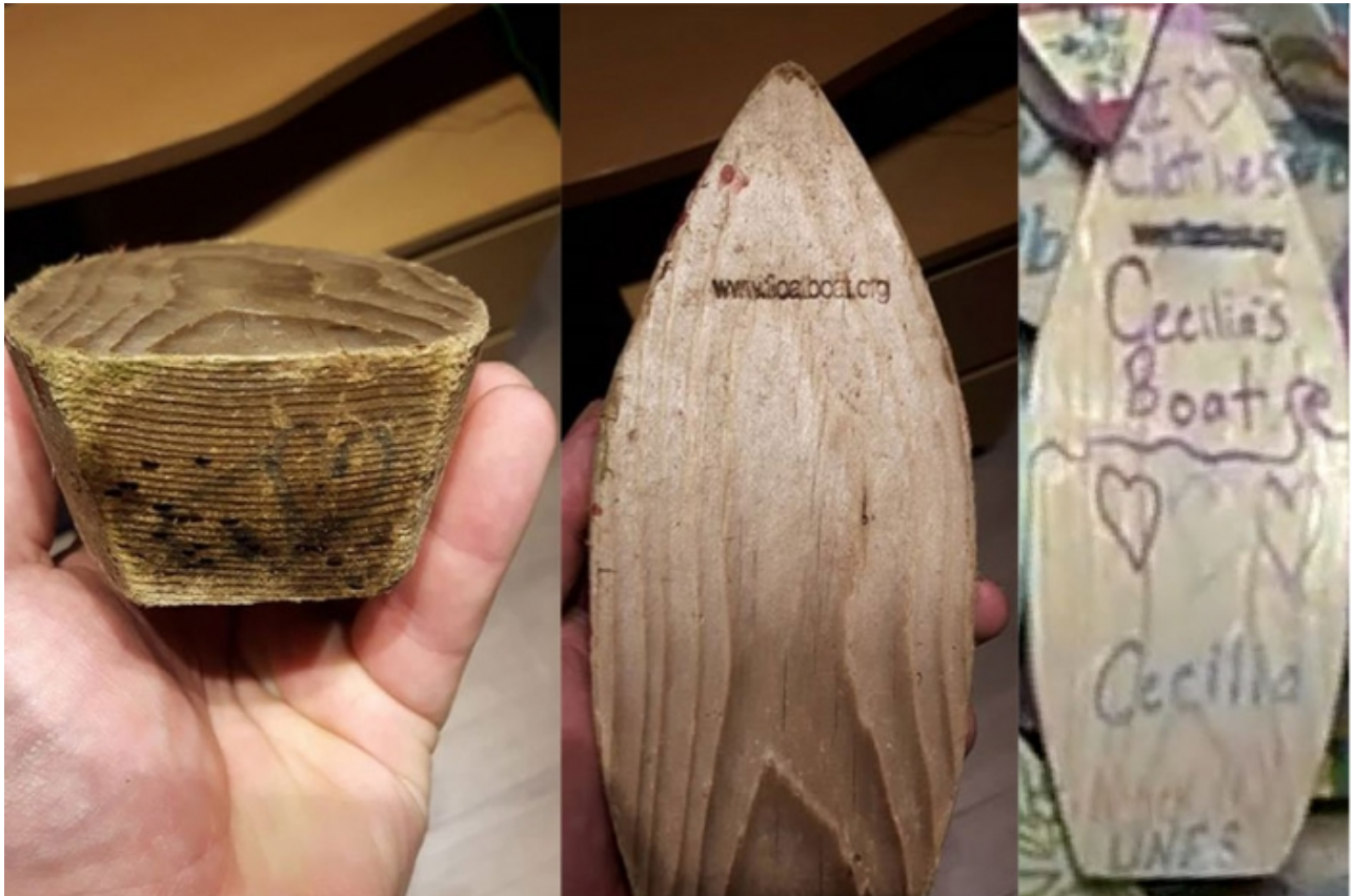
Figure 1. Left and middle: The first boat, recovered in October 2018, showing the effects of three years of weathering. Right: the boat in its original condition. Photos left and middle courtesy of Bolli Thor; photo right courtesy of the GEOTRACES Project.
