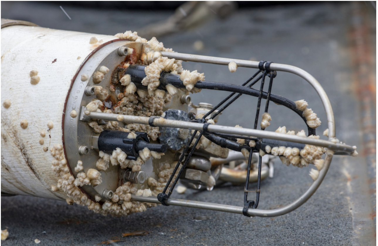
Figure 8. Barnacles growing on the casing of the hydrophone from the Chukchi Sea Ecosystem Observatory, which records the vocalizations of marine mammals and other underwater sounds. Photo courtesy of Roger Topp.
