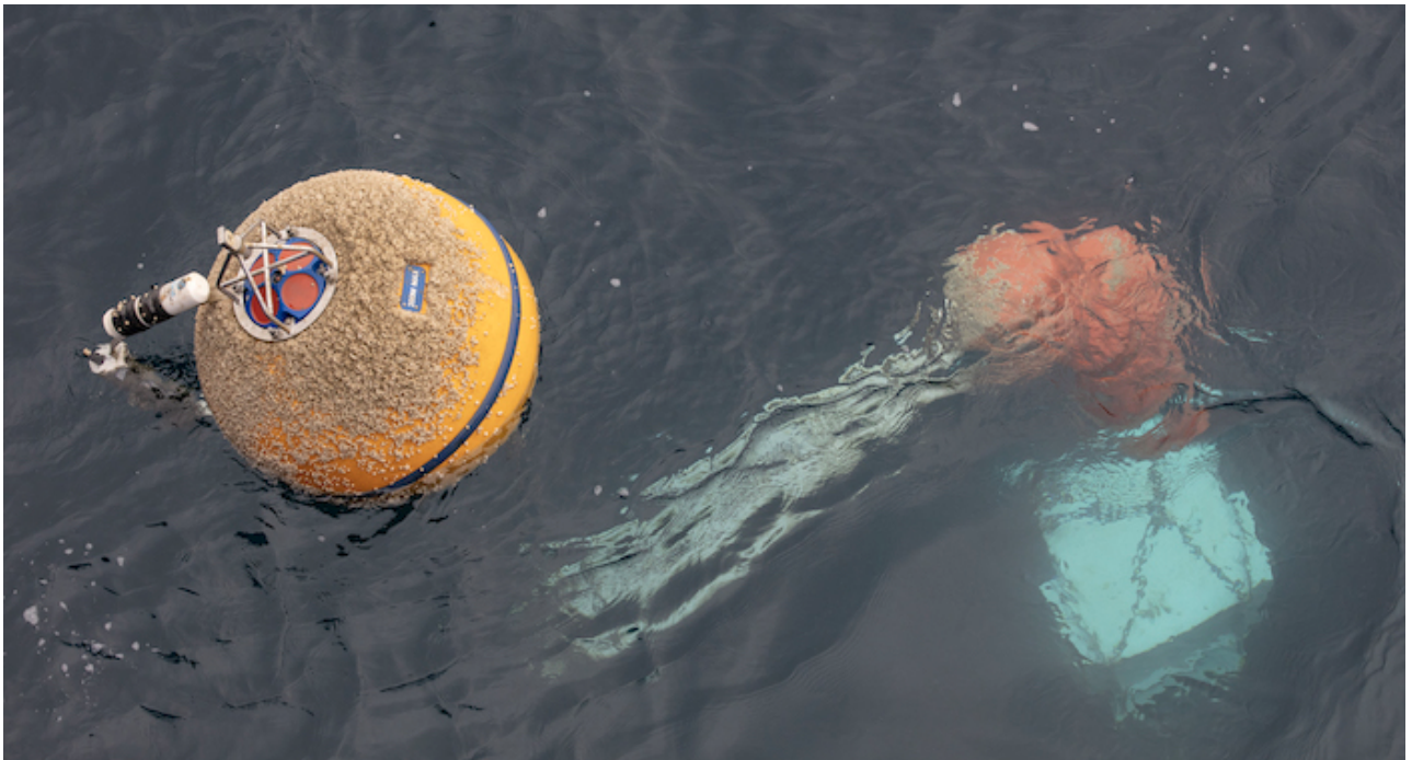
Figure 6. Recovery of a mooring from the Chukchi Sea Ecosystem Observatory showing a yellow buoy with attached acoustic Doppler current profiler, a satellite recovery beacon and a temperature/conductivity/pressure datalogger. Below the surface is a hydrophone, orange floats, and white box of the discrete water sampler, which fills IV bags with water for later laboratory chemical analyses. Photo courtesy of Roger Topp.
