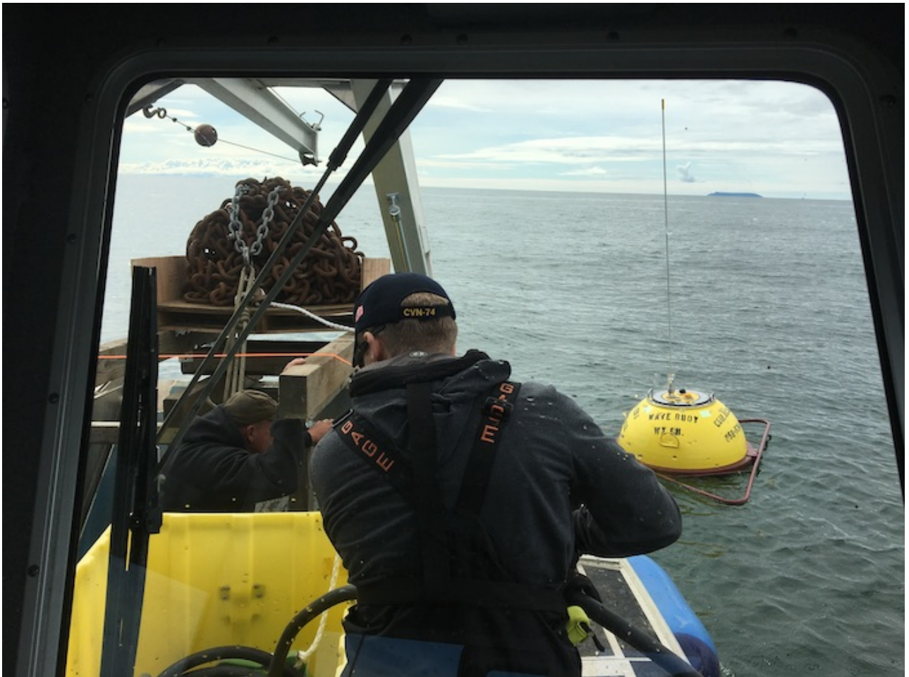
Figure 2. AOOS supported Coastal Data Information Program (CDIP) buoy being deployed off the Port of Nome in Norton Sound.
