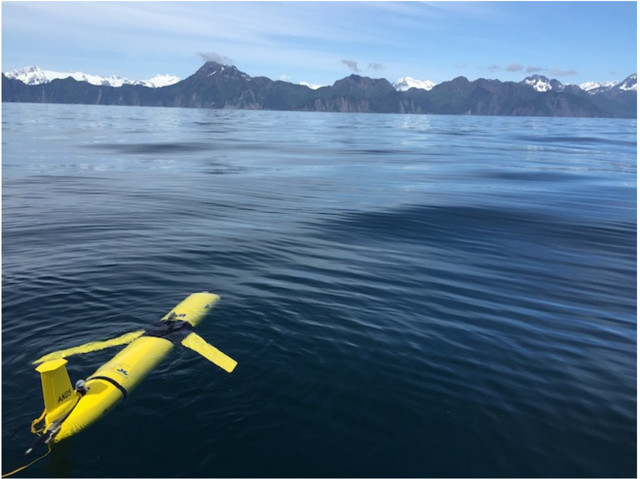
Figure 4. Deployment of AOOS funded autonomous underwater glider in the Arctic for marine mammal acoustic studies. Photo courtesy of AOOS.
