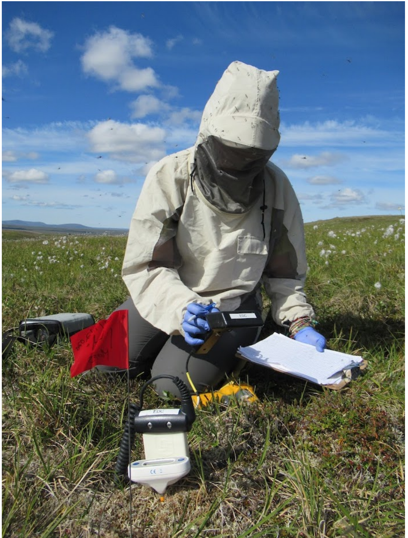
Figure 2. Kinkela Vicich, SEDC technician, recording soil properties (moisture and temperature) for a remote access MS project on examining the importance of moisture on the greenness of mosses and how that influences landscape greenness indices. Photo courtesy of Amanda Young.
