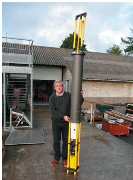
Figure 2. DAMOCLES ice-profiling float based on the MSI Provor system
