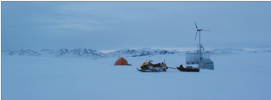
One of two solar and wind power systems currently at Imnavait Creek. As a pilot project this summer, CPS will install a methanol fuel cell at the adjacent site. The intent of the project is to improve data communications for both research sites by providing a more constant source of power while beta testing new technology in a field setting. Image by Tracy Dahl.
